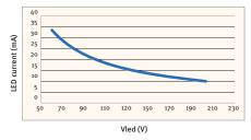
LDM200MO and LDM200MOD LED output current
